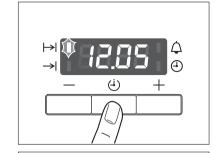
2. Using the + or — button set the desired cooking time.
